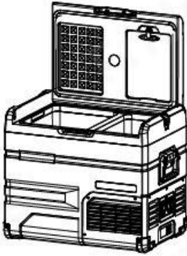
Open the door at a 90° angle
