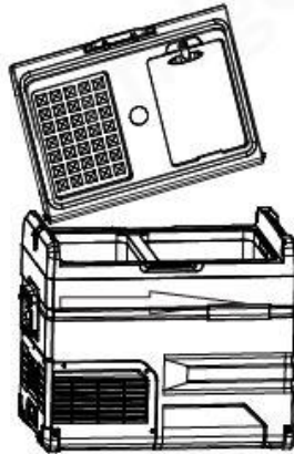
Align the door shaft with the hole on one side and insert it
