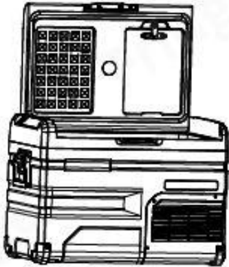
Open the door at a 90° angle
